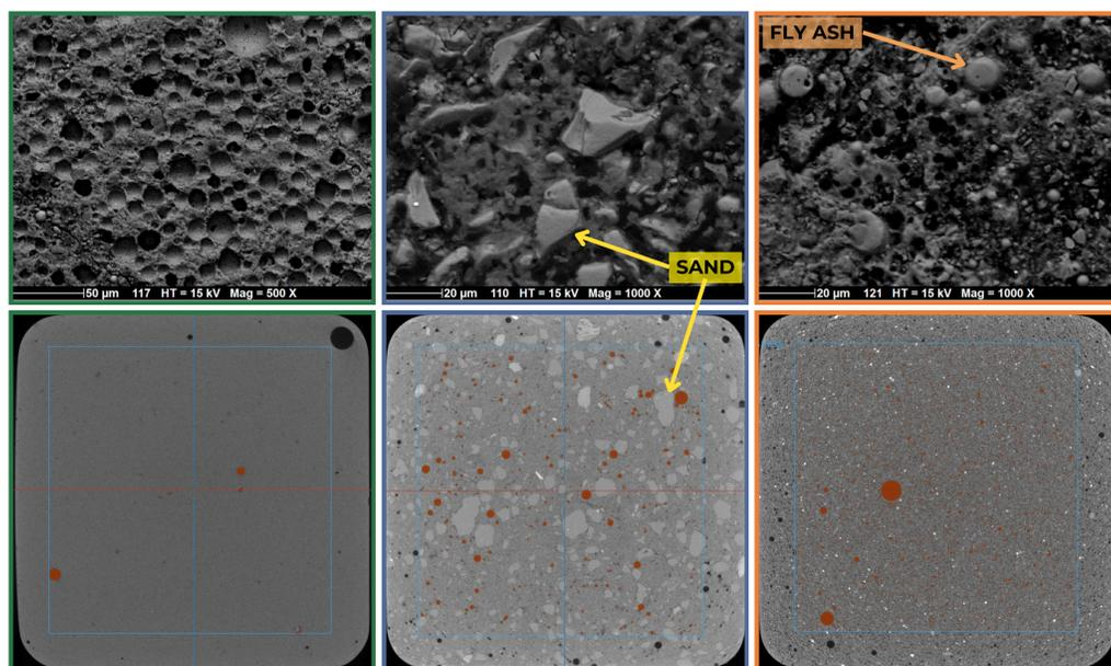
**Figure 3** - SEM (top) performed on GPs with surrogate waste. Oil pore measured less than 3  $\mu$ m. Micro-CT (bottom) performed on GPs with surrogate waste. Resolution of 15  $\mu$ m. Oil highlighted in orange.
