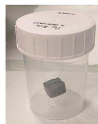
**Leaching test** was also performed to evaluate the **oil release**. A small quantity of oil was released from all three GP formulations investigated but could not be measured due to low volumes.
