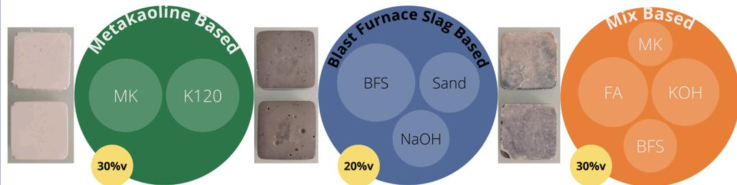
**Figure 1** - Composition of different GP studied and picture of the real samples. In the yellow circle the amount in volume of oil added.
