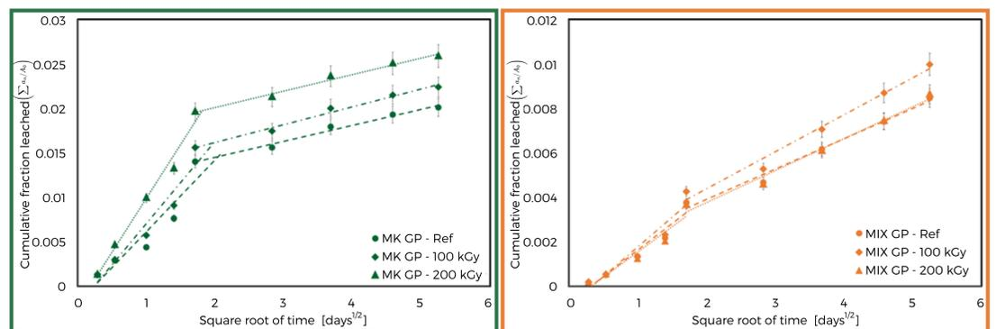
**Figure 2** - Normalised cumulative trend of Si release in leaching solution of samples without surrogate waste.
