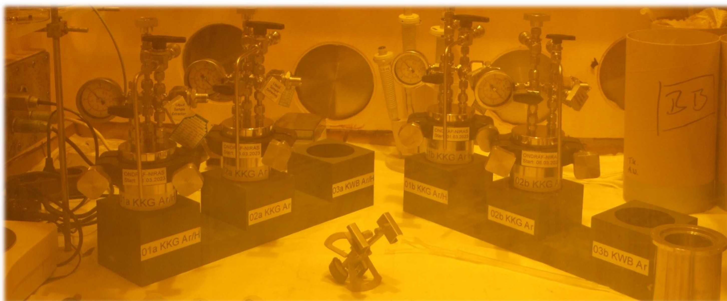
Figure 2. Examples of autoclaves in a Hot Cell at KIT-INE (Karlsruhe, Germany) used for SNF leaching experiments. Pieces of fuel rod are leached inside the pressure vessels and fluid and gas are sampled at intervals.
