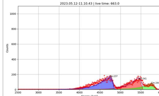
The device shows excellent spectrometric performance even at larger sourcedetector distances, despite the degraded resolution. It correctly identifies nuclides across various distances and counting statistics.
