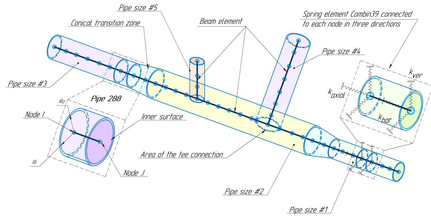
Non-linear springs in all three directions in the model for multibranch concealed piping system are used Static analysis
