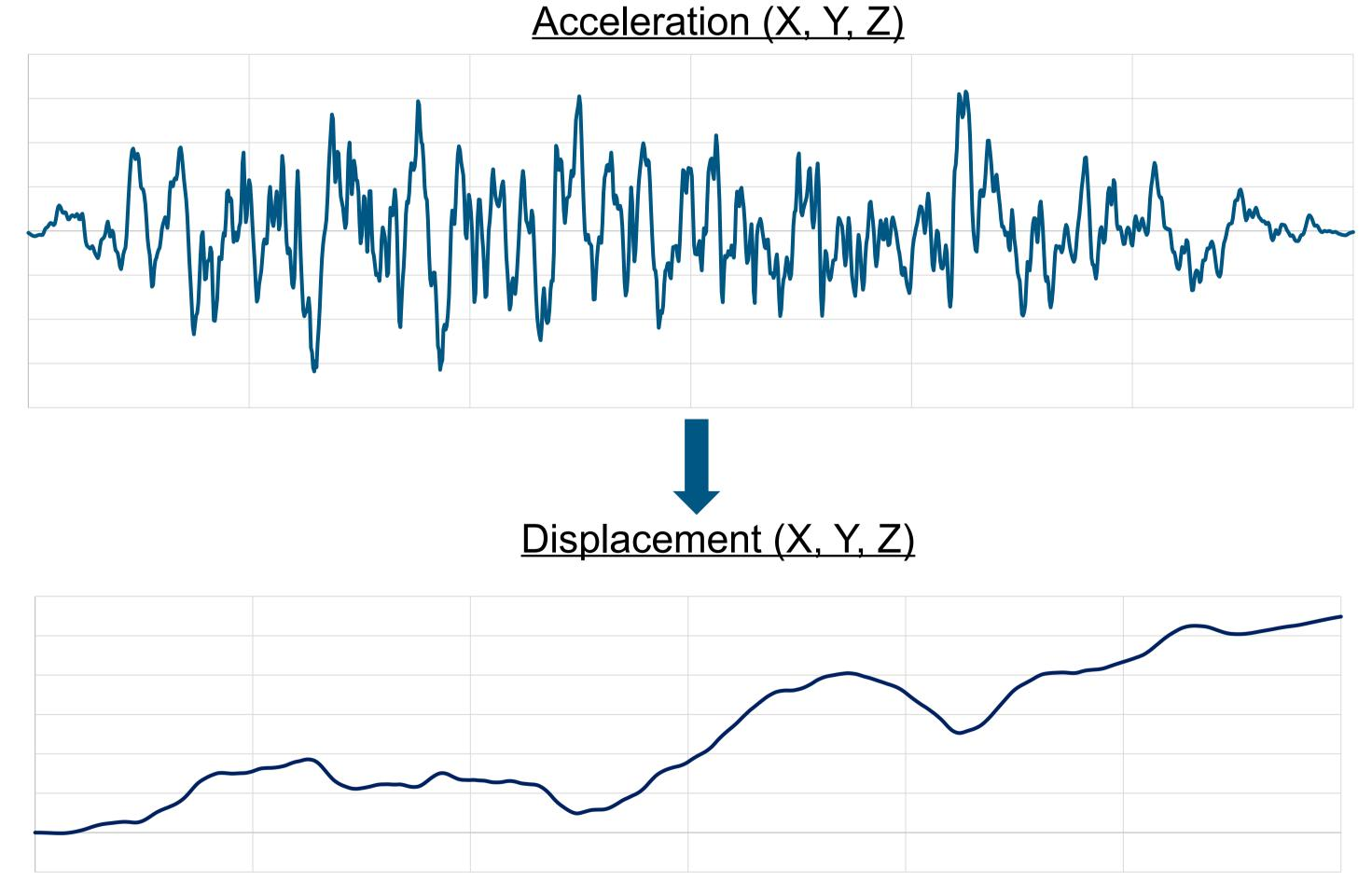
Values of permanent ground displacements at the end of oscillation process are used in stress calculation by geometrically nonlinear numerical procedure for pipe-soil interaction
