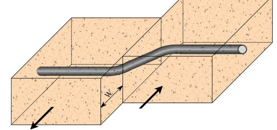
Permanent ground-induced load due to earthquakes is one of the main calculation issues for integrity assessment of the buried piping. The problem is the absence of a methodology on how to obtain the correct value of permanent ground displacement after seismic influence, depending on its magnitude.
