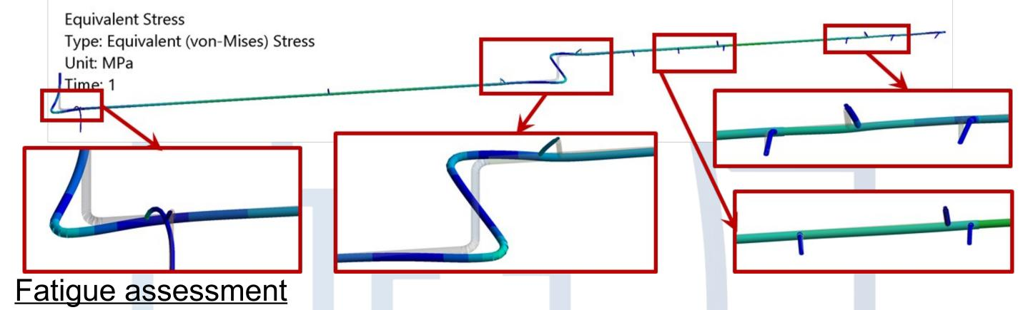
The number of load cycles for concealed piping is not regulated as a rule. During almost the entire period of operation, the piping is under normal operation conditions. Possible cycles of loading includes technical inspection every 8 years if draining for internal testing is used, seasonal water level changing, hydraulic testing.
