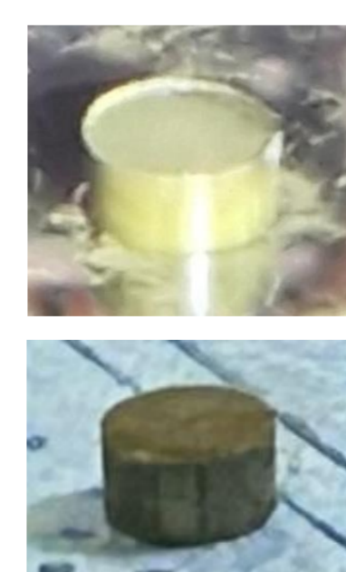
Figure 14. Photos of NpO 2 pressed pellet in different light conditions.
