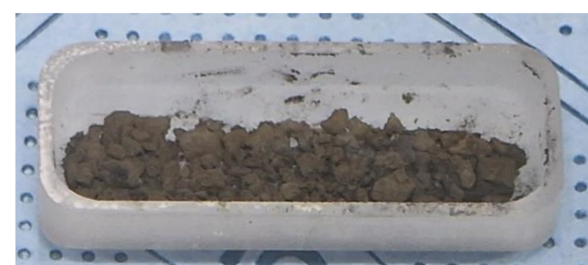
Figure 12. Hydrated Np oxalate after calcination.
