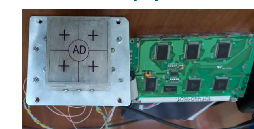
4-position alpha detector for measuring and analyzing aerosols
