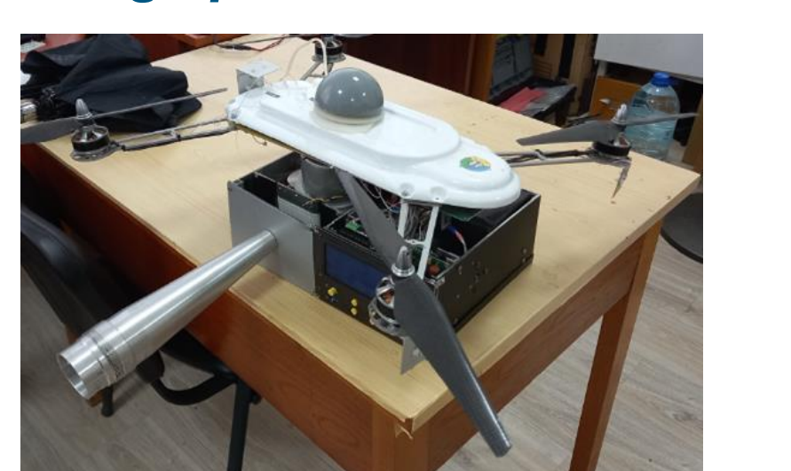
Scintillation detector with a microprocessor system for processing spectrometric data
