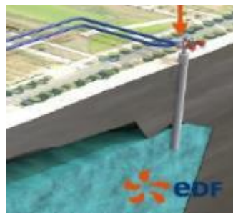
Diversified heat sink (water source for emergency supply to steam generator and fuel pool)
