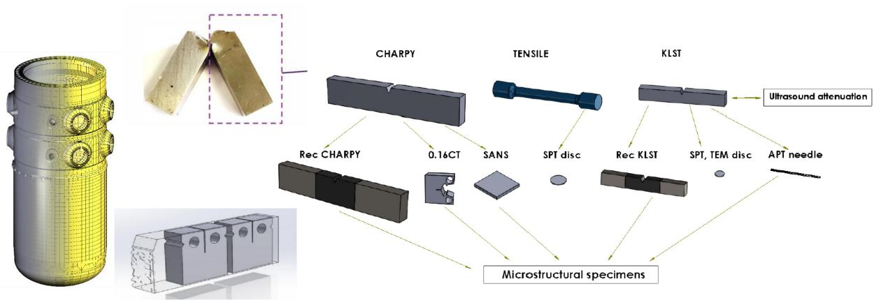
Smaller-sized specimens are developed and validated for mechanical analysis. The re-use of irradiated and fractured samples provides valuable insights into the radiation damage sustained by non-replaceable components, such as the reactor vessel, thereby supporting the extended operational lifetime of the nuclear power plant (NPP)
