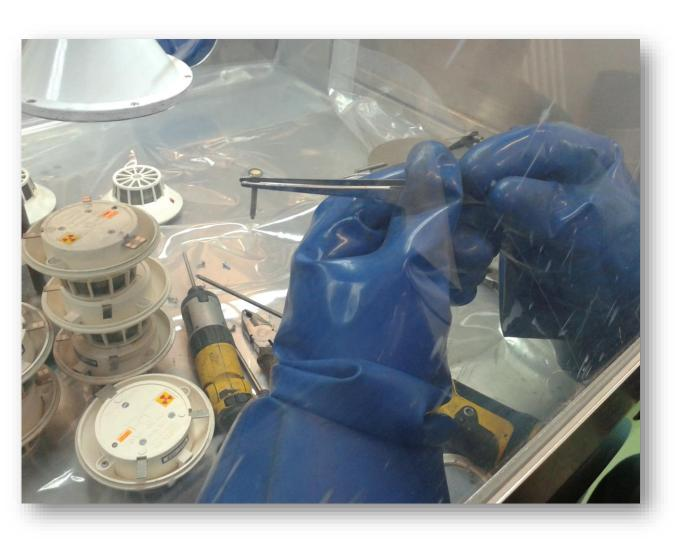
Disused Sealed radioactive sources from radioisotope smoke detectors and defectoscopes
