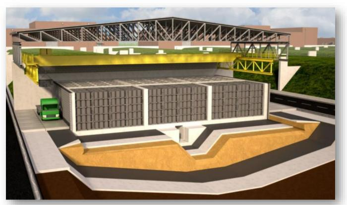
Conceptual design of a disposal facility - cross-section
